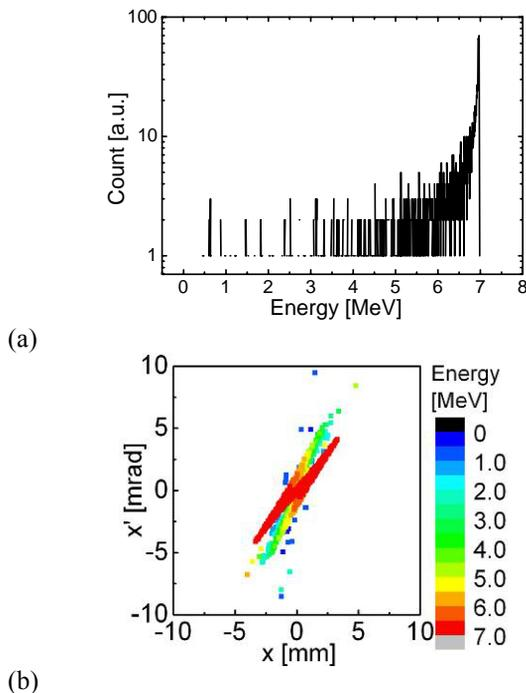
Figure 5: Realistic distribution from PARMELA at the entrance of the quadrupole magnet, (a) energy spectrum (FWHM = 0.5 % with tail), (b) phase space distribution ( $\varepsilon = 1.0\pi$  mm mrad), strongly correlated with energy distribution (the colors indicate the energy level).
