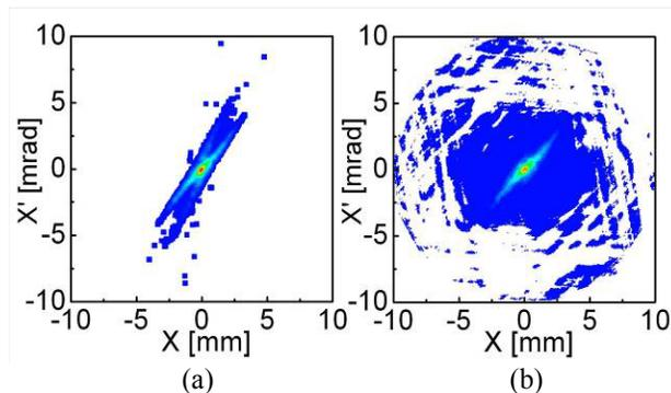
Figure 6: Phase space distributions of the realistic beam, (a) initial ( $\varepsilon = 1.0\pi$  mm mrad), (b) reconstructed ( $\varepsilon = 2.7\pi$  mm mrad)
