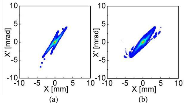
Figure 11: Phase space distributions of the realistic beam in the case of  $E_{cut-off} / E_{peak} = 70\%$ , (a) initial ( $\epsilon = 0.60\pi$  mm mrad), (b) reconstructed ( $\epsilon = 0.58\pi$  mm mrad).
