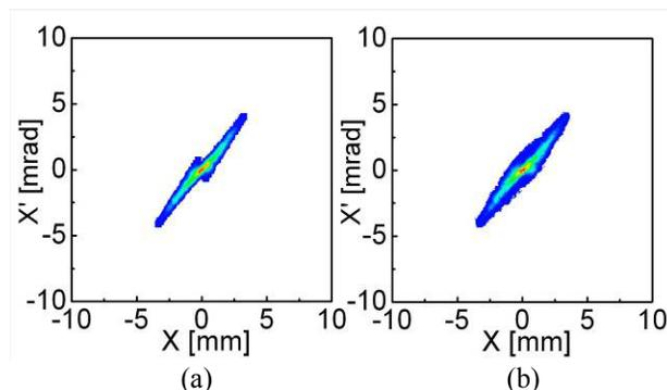
Figure 7: Phase space distributions of the realistic beam in the case of  $E_{cut-off} / E_{peak} = 90\%$ , (a) initial ( $\varepsilon = 0.43\pi$  mm mrad), (b) reconstructed ( $\varepsilon = 0.52\pi$  mm mrad).
