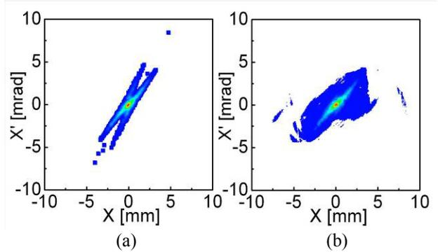
Figure 9: Phase space distributions of the realistic beam in the case of  $E_{cut-off} / E_{peak} = 50\%$ , (a) initial ( $\epsilon = 0.76\pi$  mm mrad), (b) reconstructed ( $\epsilon = 0.76\pi$  mm mrad).
