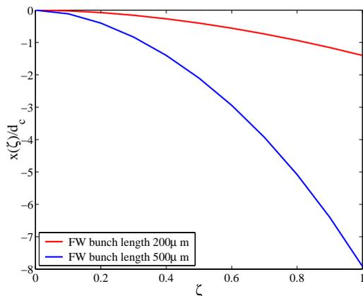
Figure 5: Normalized lateral displacements as a function of position inside the bunch at the LINAC 4 end in the short (red line) and long (blue line) bunch cases.
