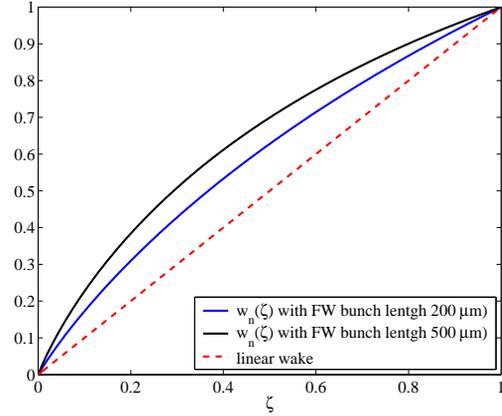
Figure 1: Comparison between wake functions (long bunch case: black line, short bunch case: blue line) and their linear approximation  $w(\zeta) = \zeta$  (red dashed line).
