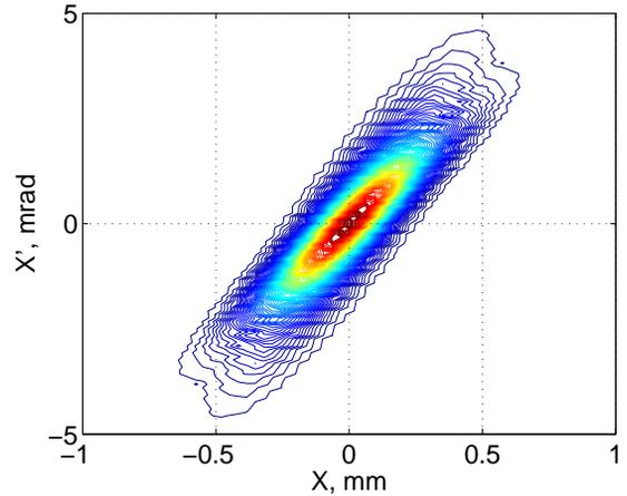
Figure 3: Reconstructed horizontal phase space based on slit scan data. The calculated 100% vertical emittance is  $\epsilon_x = 1.4$  mm mrad and the 90% core emittance is  $\epsilon_{x,90\%} = 1.0$  mm mrad. For comparison the measured 100% emittance is  $\epsilon_x = 1.3 \pm 0.1$  mm mrad.
