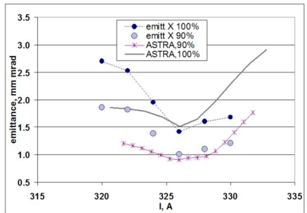
Figure 7: Estimated after phase space reconstruction 100% and 90% horizontal emittances are shown as a function of the solenoid current.
