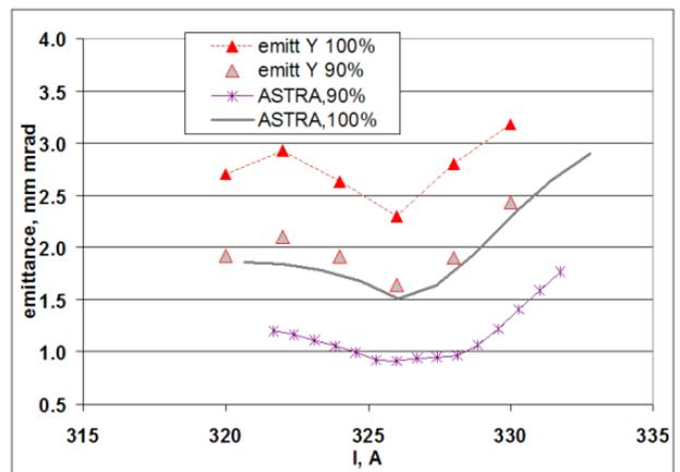
Figure 8: Estimated after phase space reconstruction 100% and 90% vertical emittances are shown as a function of the solenoid current.
