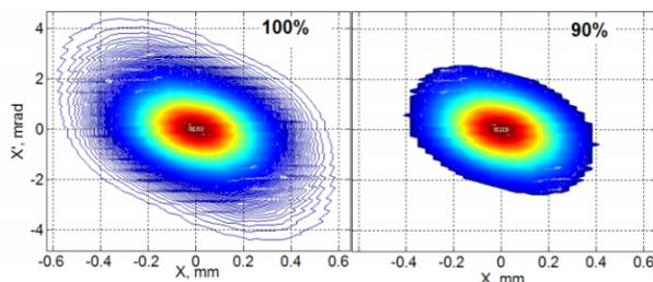
Figure 6: The figure shows the result of a thresholding of the phase space distribution. The graph in the left represents the full reconstructed distribution with an emittance of  $\epsilon = 1.95$  mm mrad. In the right the remaining points are those, where the phase space density is above a certain threshold determined so that 90% of the particles are left. The corresponding core emittance is  $\epsilon_{90\%} = 1.39$  mm mrad.
