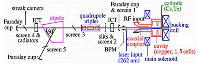
Figure 1: Schematic layout of PITZ.
