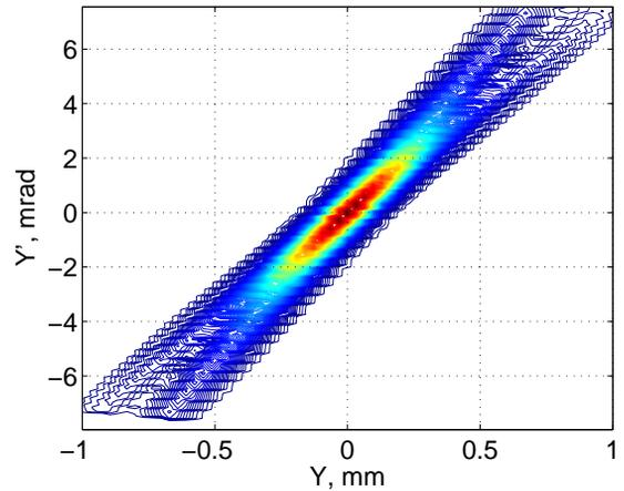
Figure 4: Reconstructed vertical phase space based on slit scan data. The calculated 100% vertical emittance is  $\epsilon_y = 2.3$  mm mrad and the 90% core emittance is  $\epsilon_{y,90\%} = 1.6$  mm mrad. For comparison the measured 100% emittance is  $\epsilon_y = 1.9 \pm 0.2$  mm mrad.
