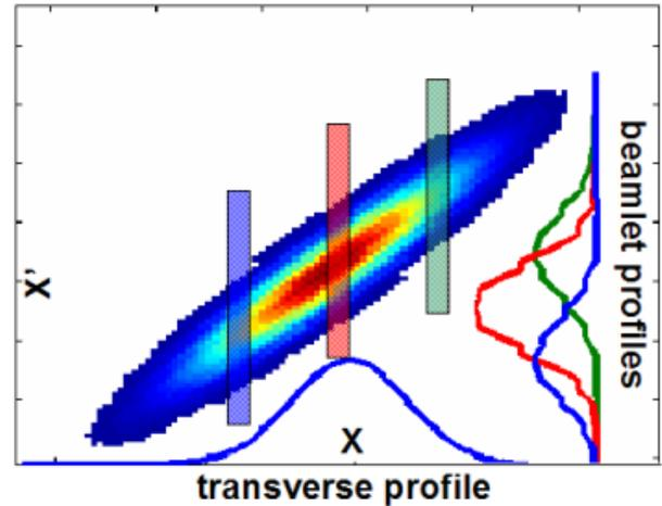
Figure 2: A schematic representation of the emittance measurement using the slit scanning technique at PITZ. The shaded stripes correspond to a phase space sampling by the slit. The beamlet profiles  $\eta_{meas}(x_i, x')$  produced by the slit are observed on a screen after about 1 m drift. The beam transverse profile  $\xi_{meas}(x)$  is measured at the position of the slit mask.
