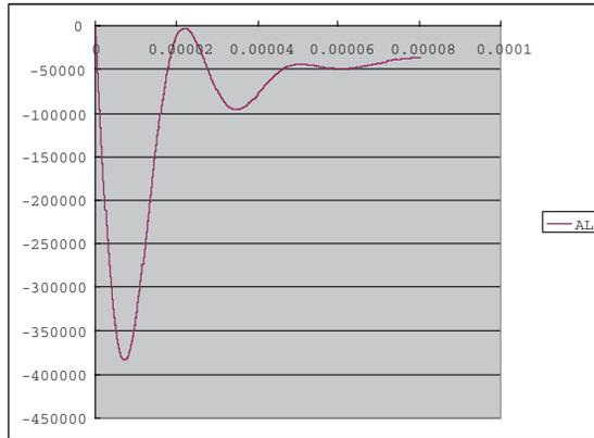
Figure 2: Wake field of a 2 mm round pipe with AL coating.
