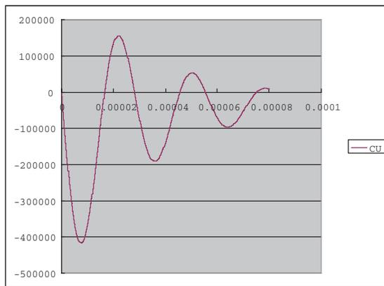
Figure 3: Wake field of a 2 mm round pipe with CU coating.
