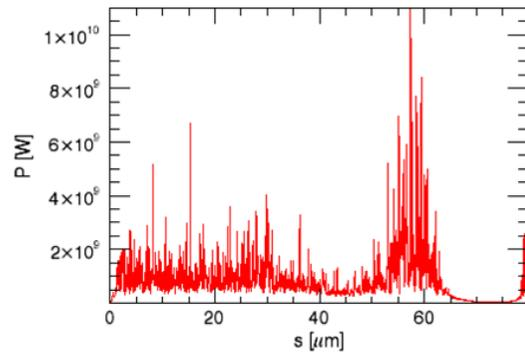
Figure 4: Time-dependent Genesis simulation over a bunch including the aluminum wake field.
