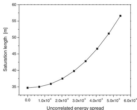
Figure 2: Saturation length as a function of the uncorrelated energy spread at the undulator entrance.
