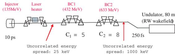
Figure 1: Layout of bunch compressors of PAL-XFEL.
