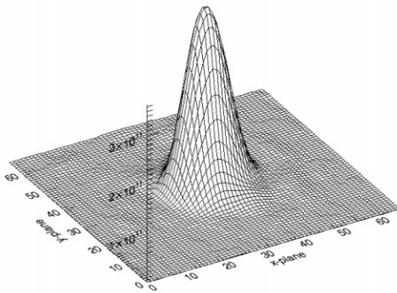
Figure 5: Radiation profile at z=80 m. The uncorrelated energy spread is 1 MeV.
