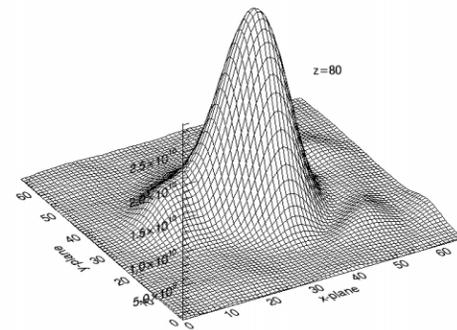
Figure 7: Radiation profile at z=80 m. The electron beam energy is 3 GeV and the uncorrelated energy spread is 1.5 MeV.
