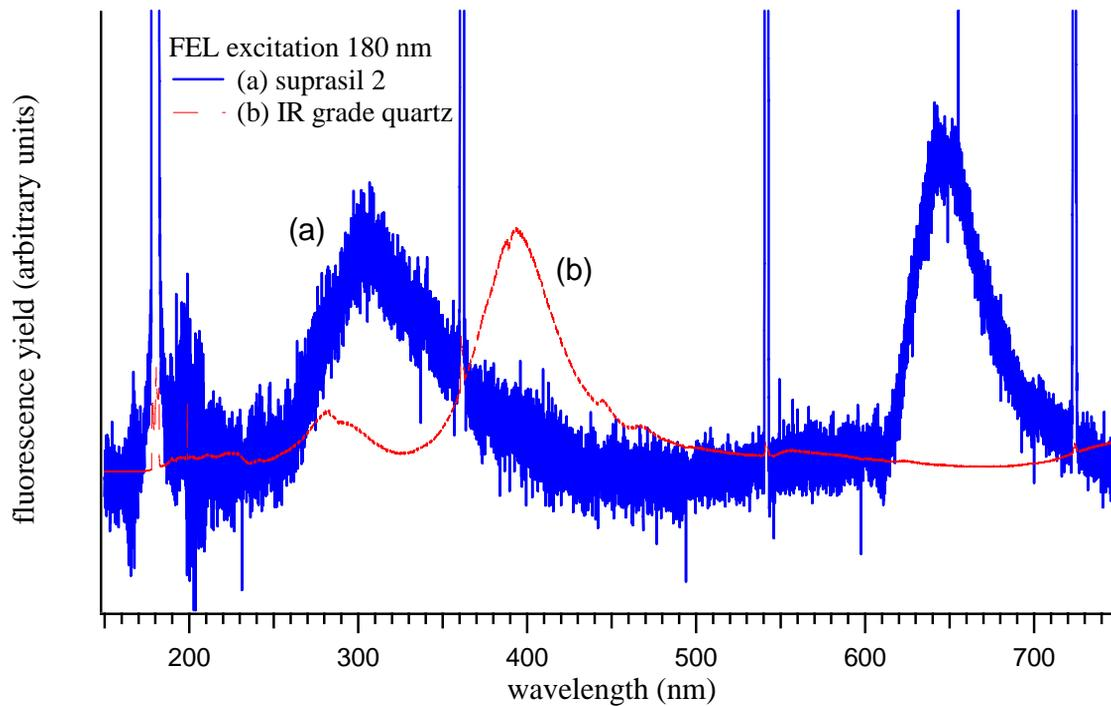
Figure 3. Fluorescence signal from suprasil 2 (a) and infrared grade quartz (b) specimens using the FEL at 180 nm as excitation source.
