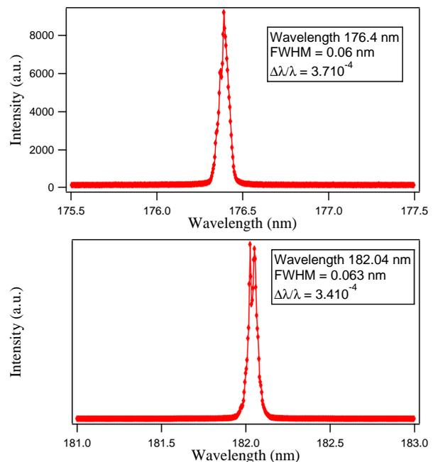
Figure 1. FEL spectra at 176 and 182 nm.
