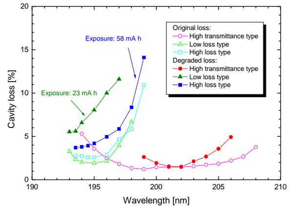
Figure 2: Cavity loss as a function of wavelength. Triangle and quadrangle represent low original-loss type and high original-loss type, respectively. For the reference, the cavity loss of the mirrors for FELs around 200 nm is shown by circle.
