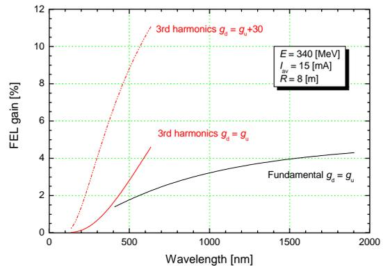
Figure 4: Relationship between the wavelength and the estimated FEL gain at the electron-beam current of 15 mA.
