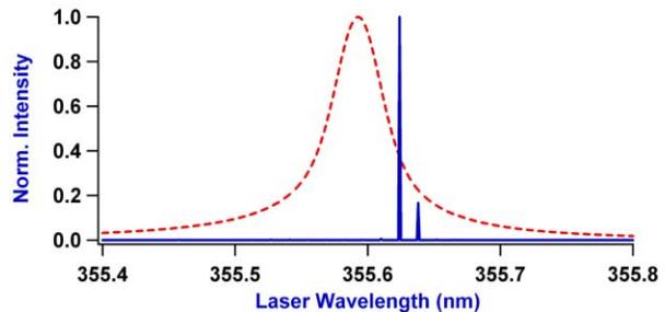
Figure 2: Results obtained on the laser spectrum with the numerical code. The dashed line shows the laser pulse without Fabry-Perot etalon, the plain line the laser pulse with the etalon
