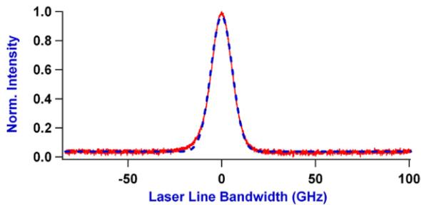
Figure 4: Laser linewidth measured by the scanning FP. The plain line is the experimental result, the dashed line is the gaussian fit.
