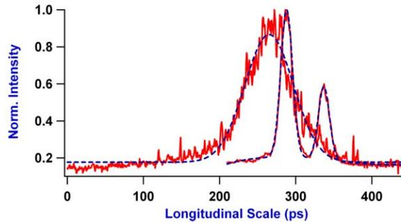
Figure 6: Results from streak camera images. The broader pulse (plain line, experiment; dashed line, gaussian fit) appears as the etalon is inserted. Ghost laser pulses appear as stray reflections, but the fits give the same result)
