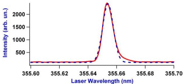
Figure 5: Laser linewidth measured by the high resolution monochromator. The plain line is the experimental result, the dashed line is the gaussian fit.
