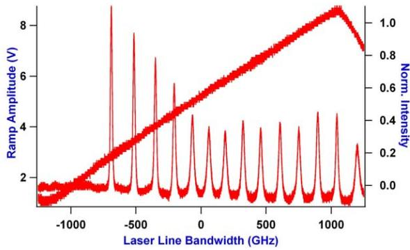
Figure 3: Operation of the Scanning Fabry-Perot. The ramp amplitude is applied on the piezoelectric motors, allowing one of the two plane mirrors to move, thus scanning several Free Spectral Ranges (in this example, the spacing between two peaks is 150 GHz, corresponding to a movement of  $\approx 650 \mu\text{m}$ )
