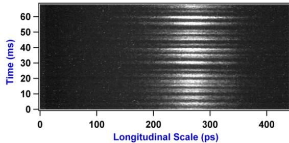
Figure 1: Image from the double sweep streak camera showing the temporal behaviour of the laser micropulse.
