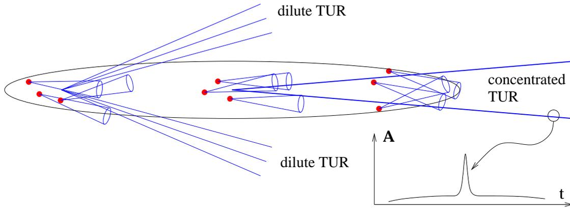
Figure 2: Schematic representation of the variations in the divergence along the bunch. The center has a smaller electron divergence, and thus a smaller TUR divergence, than the head (light rays not drawn) or the tail (divergent light rays shown). The insert shows the amplitude  $A$  over the time  $t$  at the location of the observer. Short-wavelength CTUR is due to the square of the peak over the slow pedestal.
