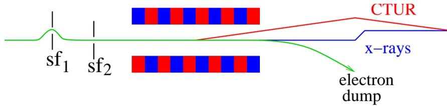
Figure 1: Schematic of the emittance-slicing scheme, with the scattering foil  $sf_1$ , as proposed in ref. [1], and the additional foils  $sf_2$  (see text). The x-rays go through a double-bounce monochromator, which has the secondary purpose of delaying them relative to the CTUR light.
