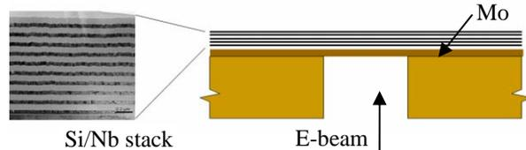
Figure 6: Diagram showing a high resolution TEM of a 100nm/60nm Si/Nb multilayer fabricated on top of a 24µm thin Mo foil supported on Al.
