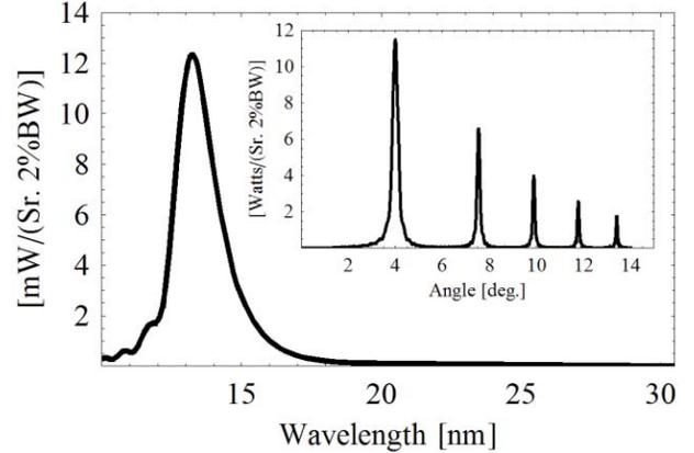
Figure 5: [MoN/Mo/MoN/vacuum]<sup>20</sup> stack (6/27/6/2100nm) emission at 7.0 MeV 0.91 mA.
