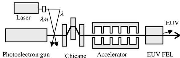
Figure 2: Schematic of the Intel FEL.
