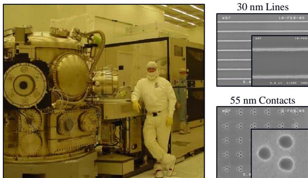
Figure 1: EUV micro exposure tool and resist images.
