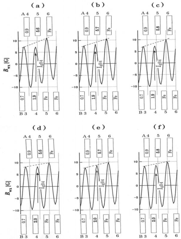
Figure 6: Partial adjustment of  $B_{wx}$  by changing the thickness of a nickel plate.
