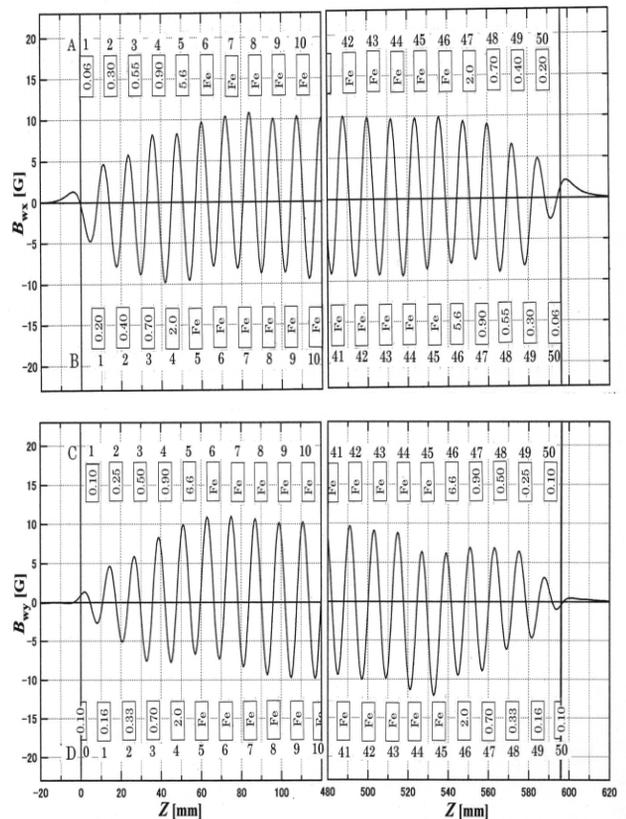
Figure 7: Measured field distribution of the wiggler.
