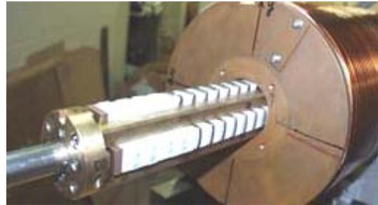
Figure 1: Adiabatic transition part of the solenoid-induced helical wiggler.
