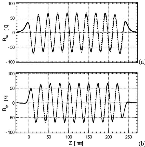
Figure 3: Simulated (solid line) and measured (dotted line) field distribution of the wiggler with a period of 24 mm.
