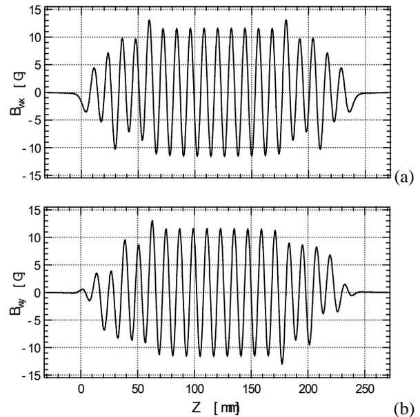
Figure 4: Simulated field distribution of the wiggler with adiabatic transition parts made of nickel plates of which each thickness is decided according to  $h_0 \sin^2(0.1\pi z / \lambda_w)$ .
