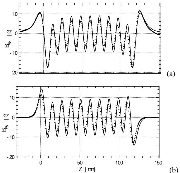
Figure 2: Simulated (solid line) and measured (dotted line) field distribution of the wiggler with a period of 12 mm.
