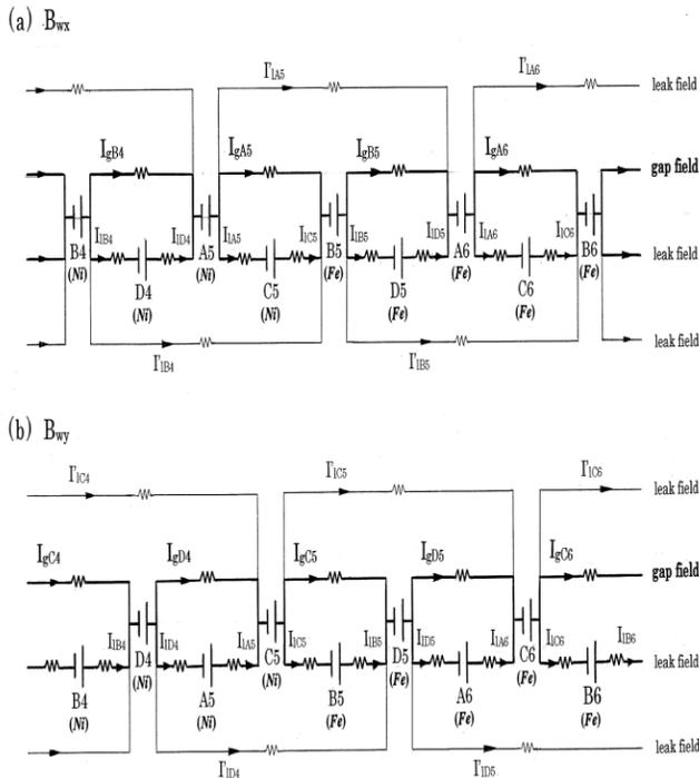
Figure 5: Schematic structure of the partial arrays of iron brocks/nickel plates, and the equivalent electric circuit for them.
