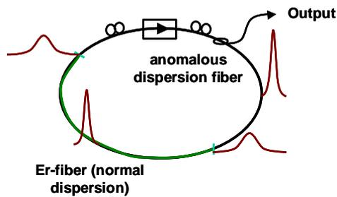
Figure 3. Schematic of the OMO, a mode-locked stretched pulse Er-fibre laser.
