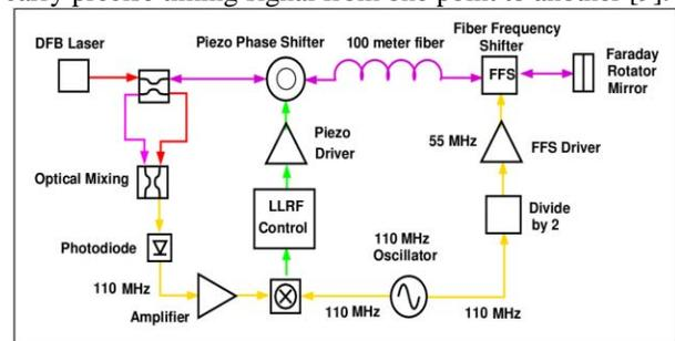
Figure 5. Scheme of the fibre stabilization set-up.
