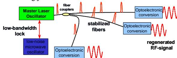
Figure 2. Conceptual schematic of the proposed MIT synchronization system.
