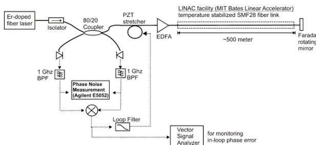
Figure 4. Schematic of the experimental setup for the synchronization experiment at the MIT-BATES facility.
