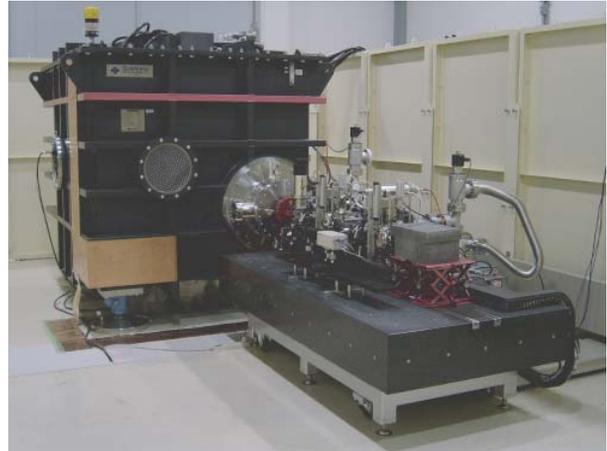
Figure 3: Prototype of an electron gun for SCSS.
