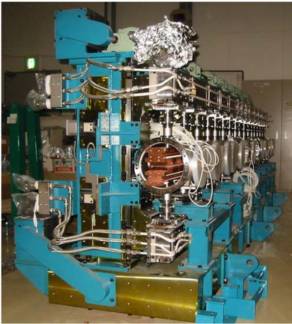
Figure 7: In-vacuum undulator for SCSS project.
