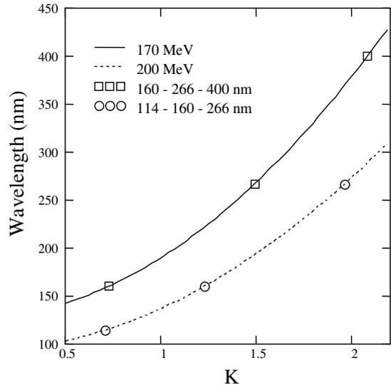
Figure 2: Seeded SPARC FEL operation wavelengths.
