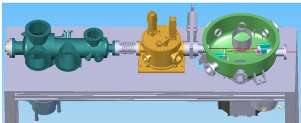
Figure 4: CATIA view of the three chambers for harmonic generation, filtering and mode matching to the undulator.
