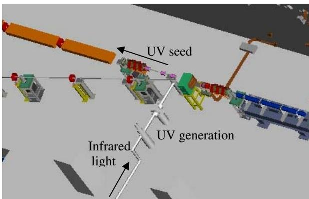
Figure 1: Seeded SPARC FEL general layout.
