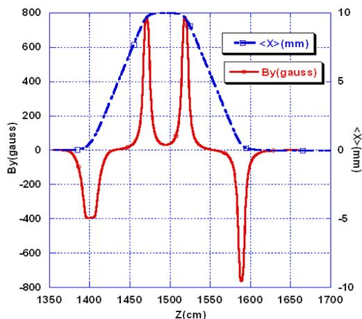
Figure 6: x-z trajectory and the  $B_y$  magnetic fields of the chicane for a bump of 10 mm at an energy of 200 MeV
