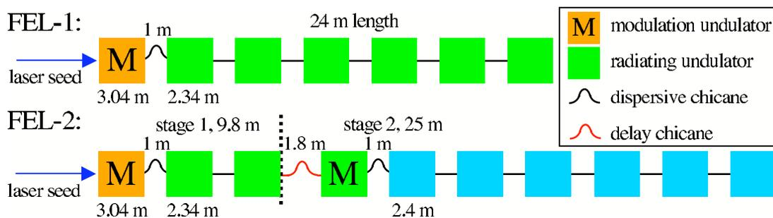
Figure 1: Layout of undulator beamlines for FEL-1 and FEL-2.
