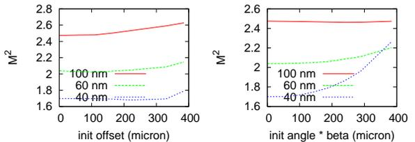
Figure 6: Plot of  $M^2$  as a function of initial displacement (left) and tilt (right), for FEL-1 at 100, 60, and 40-nm wavelengths. Tilts are normalized to the beta function. Data are from *GENESIS* simulations.
