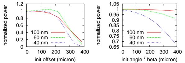
Figure 5: Plot of power reduction due to initial displacement (left) and tilt (right), for FEL-1 at 100, 60, and 40-nm wavelengths. Tilts are normalized to the beta function. Data are from *GENESIS* simulations.
