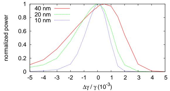
Figure 9: Plot of power reduction due to variation in electron beam energy for FEL-2 at 40, 20, and 10-nm wavelengths. Data are from *GENESIS* simulations.
