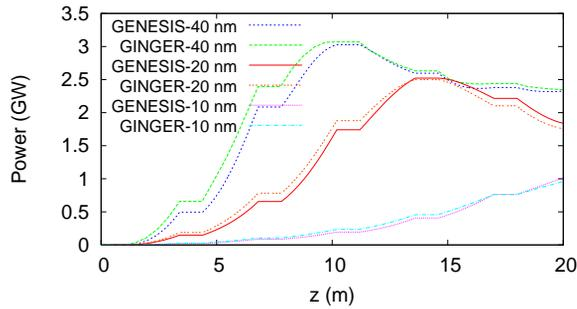
Figure 7: Plot of power vs.  $z$  for FEL-2 at 40, 20, and 10-nm wavelengths. Comparison of *GINGER* and *GENESIS* simulation results.
