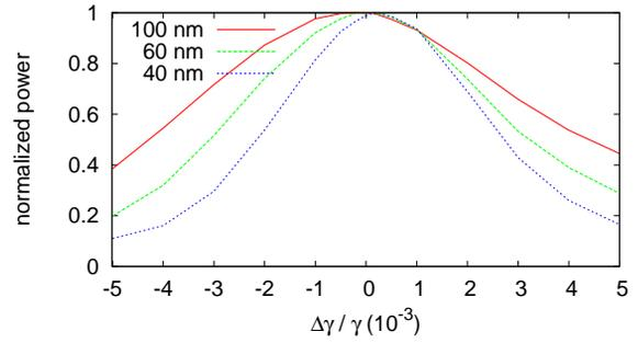
Figure 4: Plot of power reduction due to variation in electron beam energy for FEL-1 at 100, 60, and 40-nm wavelengths. Data are from *GENESIS* simulations.
