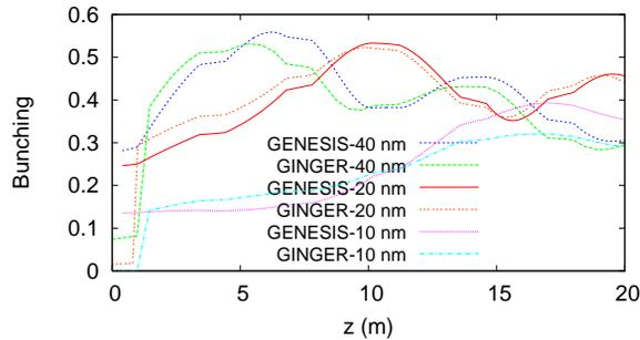
Figure 8: Plot of bunching vs.  $z$  for FEL-2 at 40, 20, and 10-nm wavelengths. Comparison of *GINGER* and *GENESIS* simulation results.
