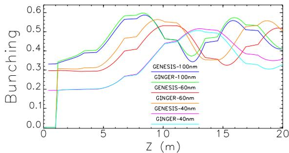
Figure 3: Plot of bunching vs. z for FEL-1 at 100, 60, and 40-nm wavelengths. Comparison of *GINGER* and *GENESIS* simulation results.
