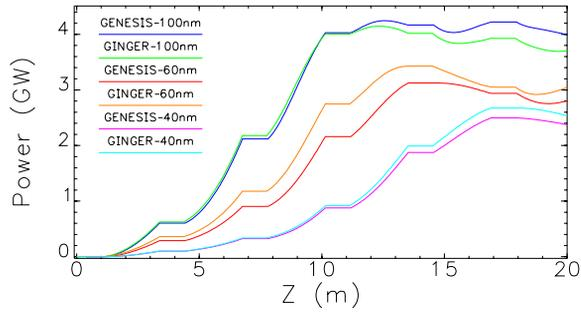
Figure 2: Plot of power vs. z for FEL-1 at 100, 60, and 40-nm wavelengths. Comparison of *GINGER* and *GENESIS* simulation results.
