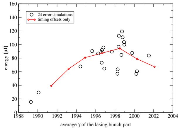
Figure 3: Pulse energy as a function of the averaged  $\gamma$  of the radiating bunch part in the final amplifier for 24 bunches.  $\gamma$  is proportional to the arrival time.
