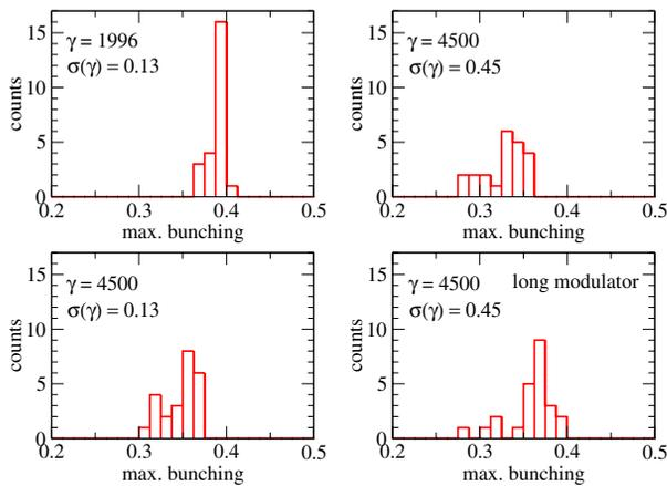
Figure 5: Histograms of the maximal bunching yielded after the first modulator and dispersive section: Top left: Low energy FEL line. Top right: Medium energy line (ME), high energy spread. Bottom left: ME, low energy spread. Bottom right: ME, high energy spread, but long modulator.
