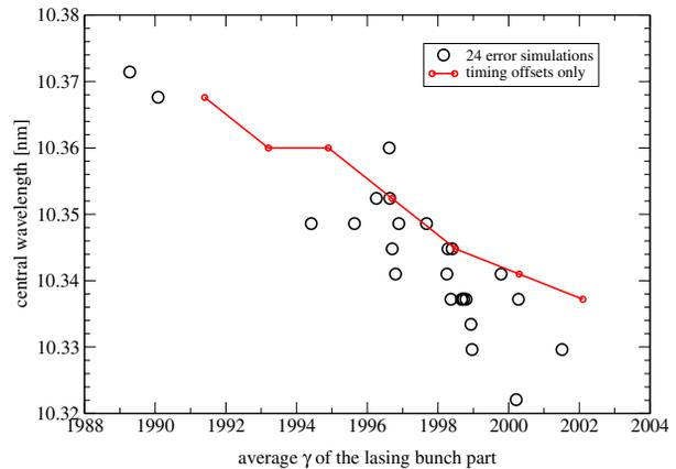
Figure 4: Central wavelength as a function of the averaged  $\gamma$ . A reduction in the arrival time jitter would reduce the spread in the wavelengths.
