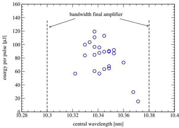
Figure 2: Energy per pulse as a function of the central wavelength delivered by the final amplifier in the low energy FEL line for 24 error simulations.
