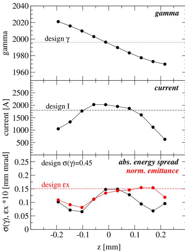
Figure 1: Parameter profile of the bunch at the beginning of the low energy FEL line, when no errors are applied. The profiles are similar for the ME-FEL at  $\gamma = 4500$ . seeding radiation.
