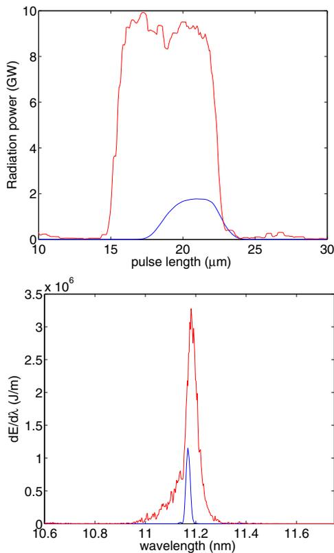
Figure 6: Temporal and spectral power distribution of fifth harmonic radiation pulse for optimized all-helical undulator, red, compared to nominal stage two radiator output, blue. Strong focusing applied along radiator to conserve bunching.
