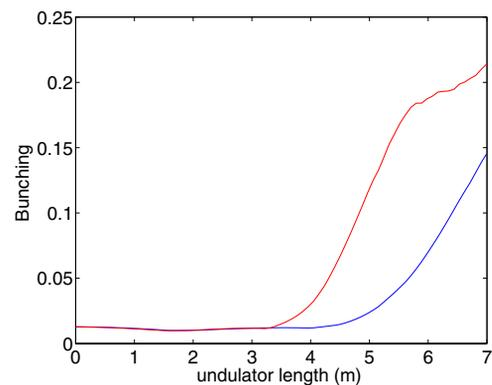
Figure 5: Evolution of fifth harmonic bunching in first stage radiator when using planar undulator, blue, or helical undulator, red.
