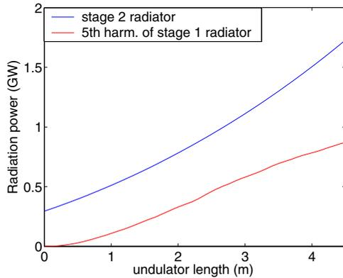
Figure 1: Evolution of peak power of fifth harmonic radiation in first stage radiator with optimized undulator  $K$  parameter, red line.  $K$  changed by 0.3% of its nominal value. Results are compared to peak pulse power in original stage two radiator, blue line, with same resonant wavelength 11.18 nm.
