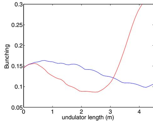
Figure 2: Evolution of bunching on fifth harmonic along extended radiator for nominal electron beam size, blue, and optimized electron beam size, red.
