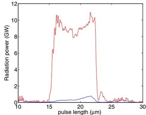
Figure 4: Temporal power distribution of fifth harmonic radiation at radiator end when last radiator part is helical. Compared are power for nominal electron beam size, blue, and optimized beam size, red.
