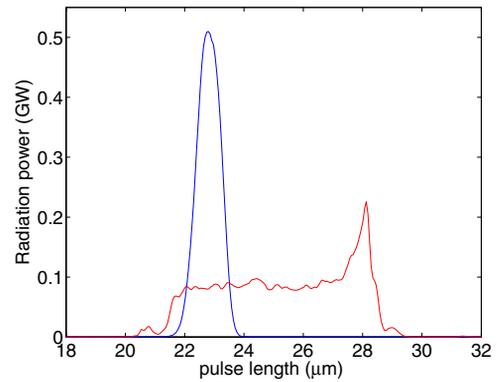
Figure 7: Radiation pulse at end of third radiator when using fifth harmonic radiation of first radiator as a seed. Compared are the powers that can optimally be achieved using all planar undulators, blue, or helical undulator, red.
