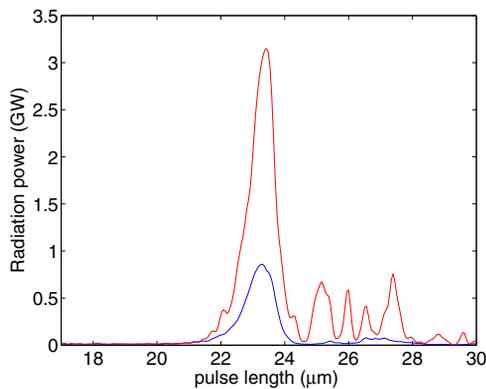
Figure 3: Temporal power distribution of fifth harmonic radiation at radiator end for nominal electron beam size, blue, and optimized electron beam size, red.
