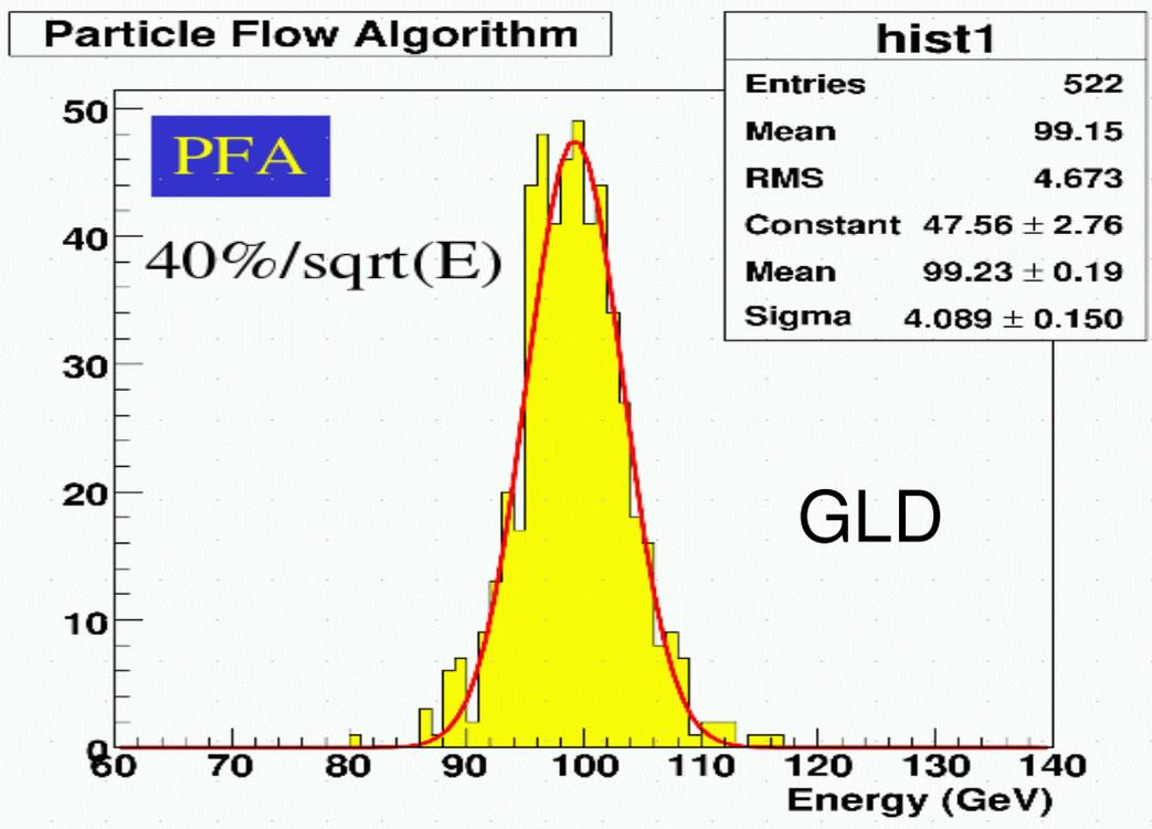
Results obtained by different groups for SiD, LDC and GLD are comparable ( $dM/M \sim 40\%/sqrt(M)$ )
