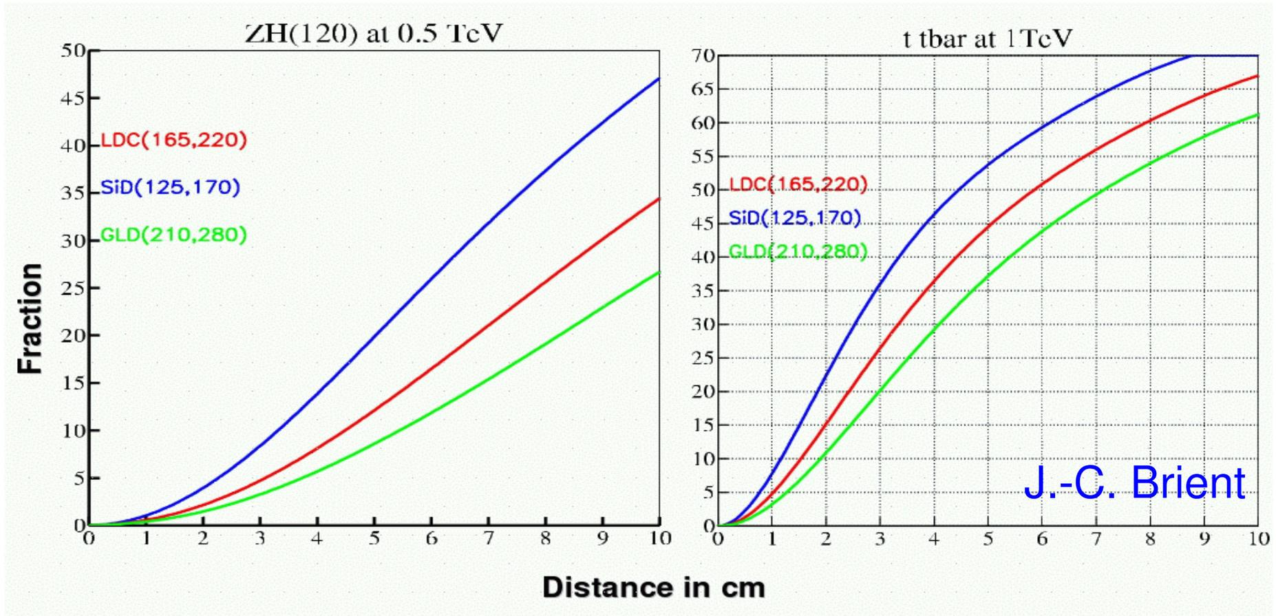
Efficient separation of photons from charged particles requires highly granular ECAL ( cell size  $\leq 1 \times 1 \text{ cm}^2$ )
