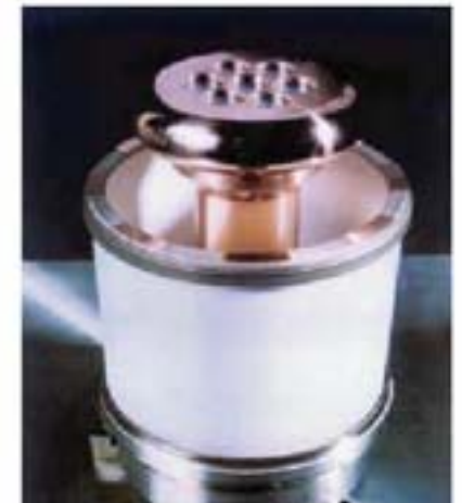
Photo of TH1801 Tube (top) and Cathode (bottom)
