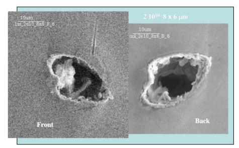
Electron micrograph of single electron bunch "silhouette of passage" through 0.25 RL Cu target; courtesy of Doug McCormick, SLAC
