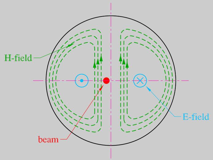
Principle of a cavity BPM.
