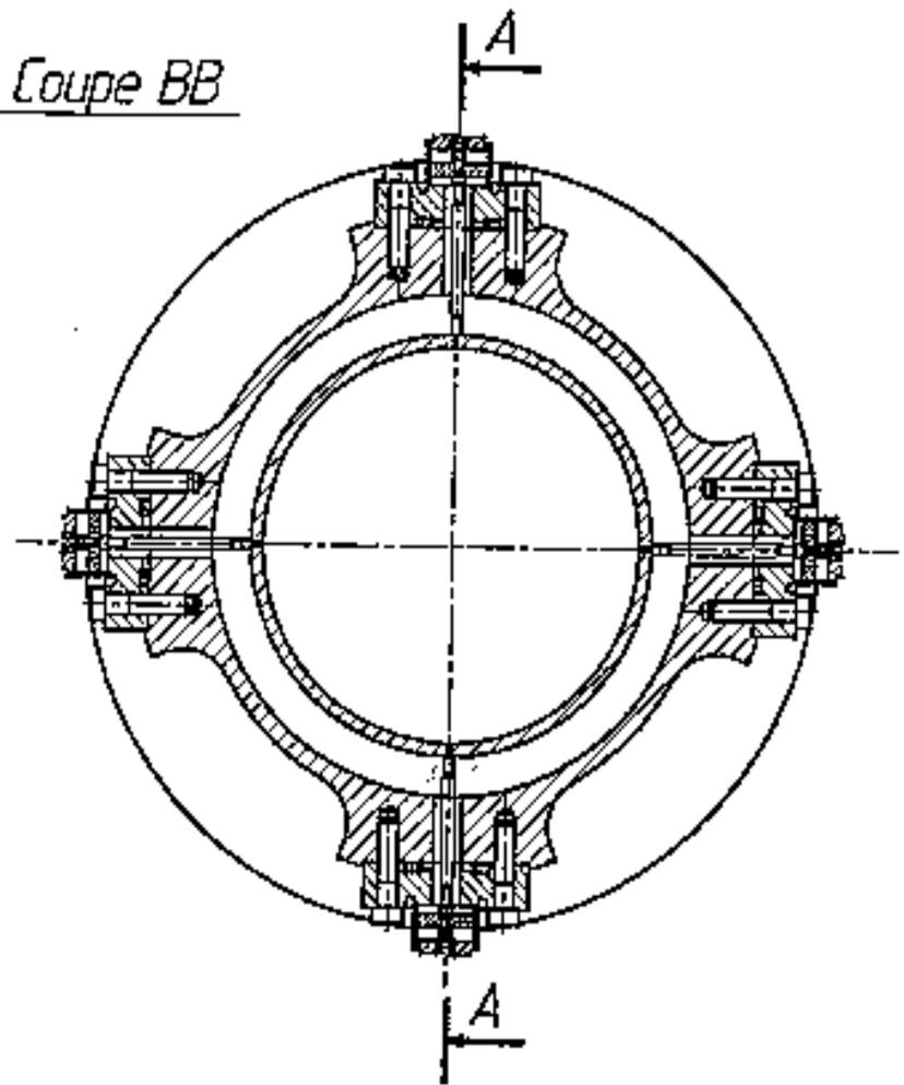
Re-entrant coaxial-cavity BPM for TTF2.
