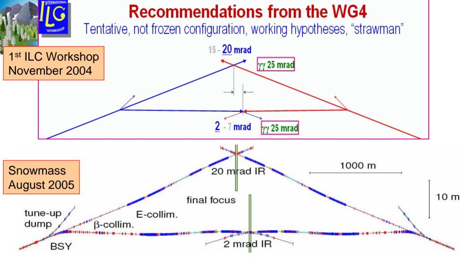
Strawman tentative configuration turns into real design: Full optics for all beamlines; Mature 20mrad optics and magnets design; Several iteration of optics for 2mrad IR; Upstream and downstream diagnostics for both IRs Baseline: two BDSs, 20/2mr, 2 detectors, 2 longitudinally separated IR halls
