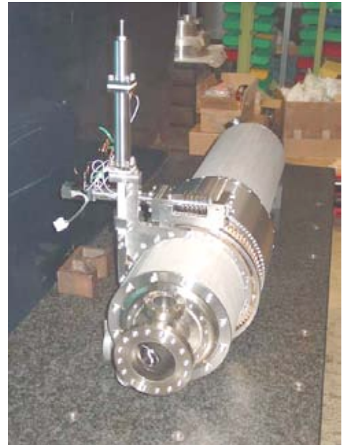
Coaxial ball-screw tuner on ICHIRO 2nd 9-cell cavity
