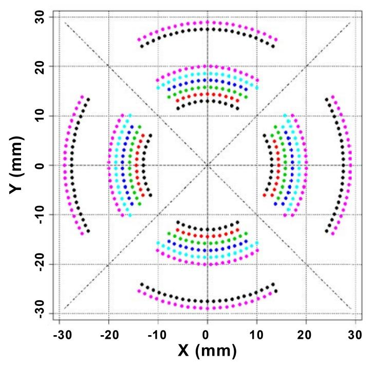
For compensation  $G_{in}$  = 160 T/m at  $I_o$  = 767 A  $G_{out}$  = -20 T/m at  $I_o$  = 517 A for  $G_{eff}$  = 140 T/m  $L_{mag}$  = 2.200 m  $L_{coil}$  = 2.228 m
