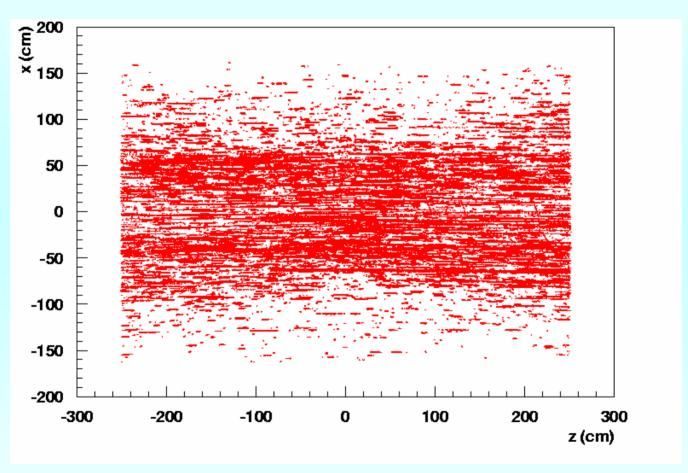
Larger opening angle of the mask results in more backscattering into the TPC
