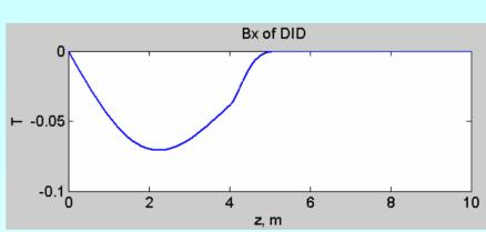
DID field combined with FD offset to zero both angle and position at the IP
