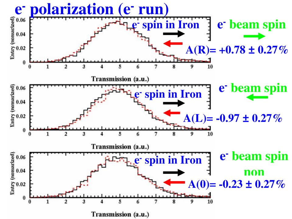
**Summary of Experiment** 1) The experiment was successful. High intensity short pulse polarized e<sup>+</sup> beam was firstly produced. **Pol.** ~ 80% 2) We confirmed propagation of the polarization from laser photons -> -rays -> and pair created e<sup>+</sup>s & e<sup>-</sup>s. 3) We established polarimetry of short pulse & high intensity -rays, positrons, and electrons.
