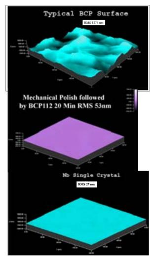
RMS: 1274 nm fine grain bcp 53 nm after ~ 35 micron, single Crys 27 nm after ~ 80 micron, single Crys 251 nm fine grain ep
