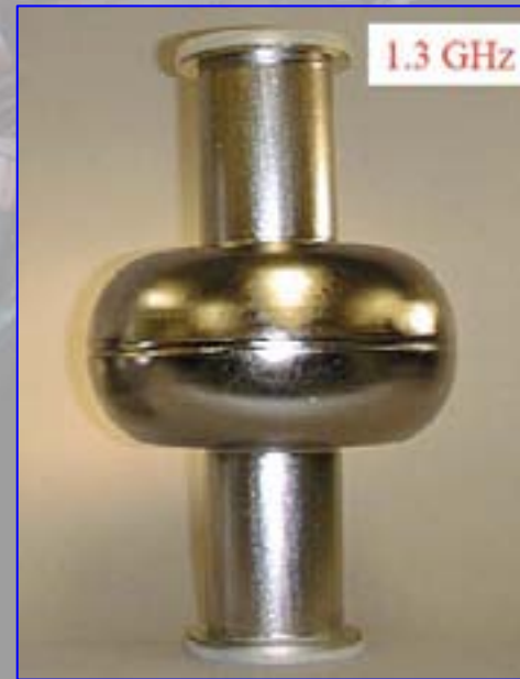
Re-entrant cavity shape is shown. Taken from Rong-Li Geng SRF 2005
