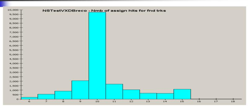
We should expect 10 hits for high Pt low cos(theta) tracks and 15 hits for low Pt high cos(theta) (traversing all 10 endcap silicon strip layers). Very small amount of tracks with more than 15 hits is due to tracks hitting most of barrel layers, and traversing almos all endcaps – this is possible for narrow region of phase space)
