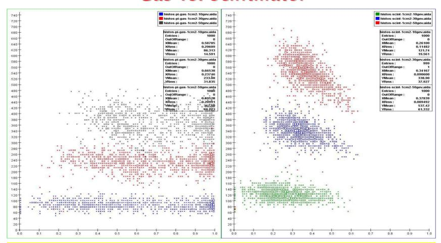
2-bit readout affords significant resolution improvement over 1-bit for scintillator, but not for gas
