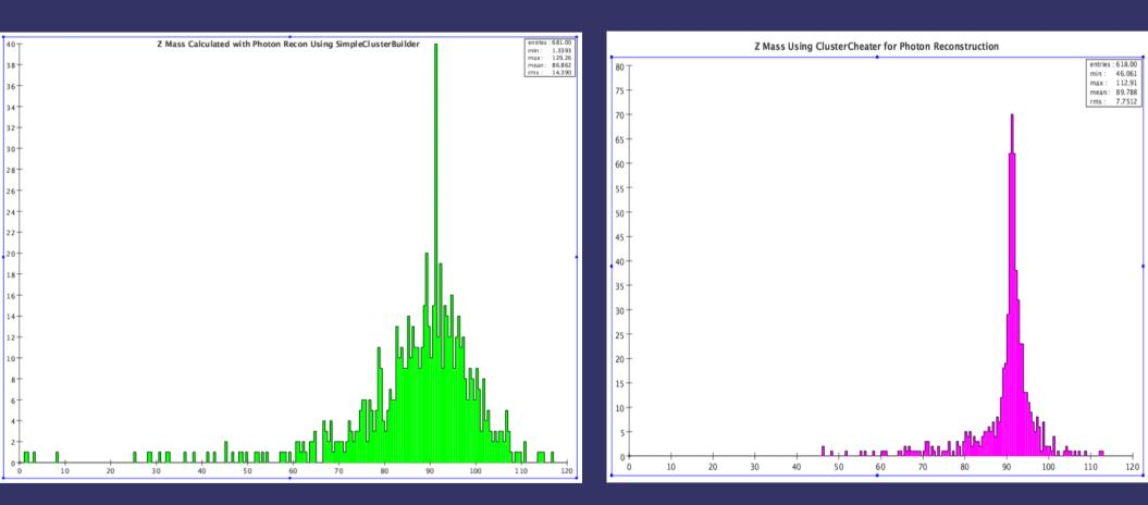
Because of the more efficient photon reconstruction using CC, the Z mass peak is much less sloppy and is shifted up.
