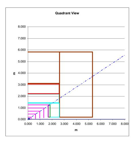
Rtracker = 1.25 m  $Cos(\Theta_{barrel}) = 0.8$ B = 5 T Cal radiators are W Hcal 4A, 2X<sub>0</sub> (7mm)
