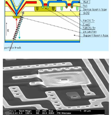
Integration of a fully depleted p<sup>+</sup>-n junction matrix and the readout electronics in a wafer bonded SOI substrate
