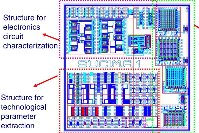
Detector prototypes (8x8 pixels) w/ and w/o charge injection pad.
