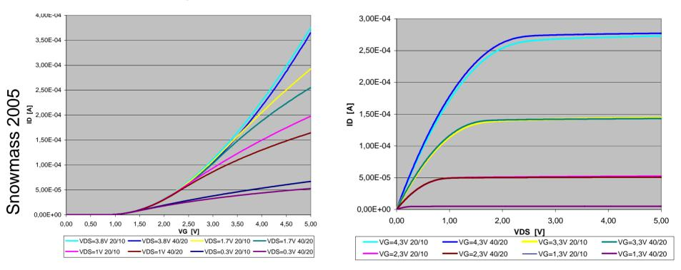
$g_{ds} \approx 428 \text{ nS} @ V_{GS} = 2.3 \text{ V} \text{ for W/L} = 20/10$  $g_{ds} \approx 196 \text{ nS} @ V_{GS} = 2.3 \text{ V} \text{ for W/L} = 40/20$
