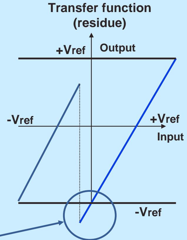
Missing codes due to comparator offset for example
