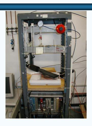
Test 8x8 cm<sup>2</sup> area defined by two scintillator trigger counters.
