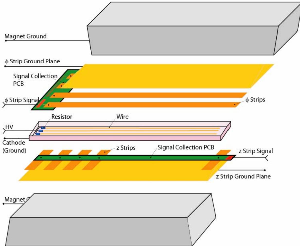
One can read out the  $z$  and  $f$  coordinate of the hit through the strips in both direction but for our case, the  $\phi$  signal is read through the anode wire rather than  $\phi$ -strips
