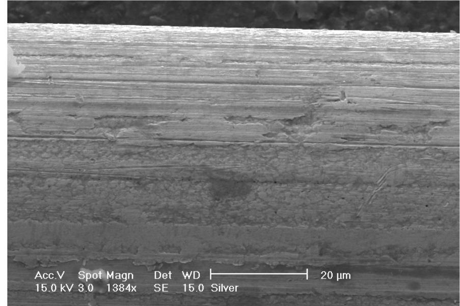
**Surface quality looks similar to the Au-coated wire. Use SEM scale measured wire diameter is 107μm. Micrometer measured diameter is 105μm.**
