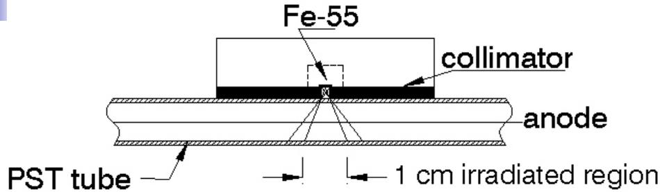
**X-ray irradiation distribution along anode wire direction**
