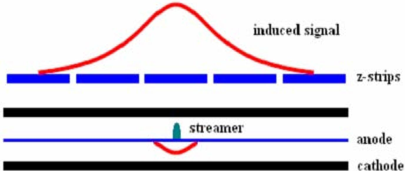
Segmented strips adjacent to detector pick up induced charge signal from the streamer
