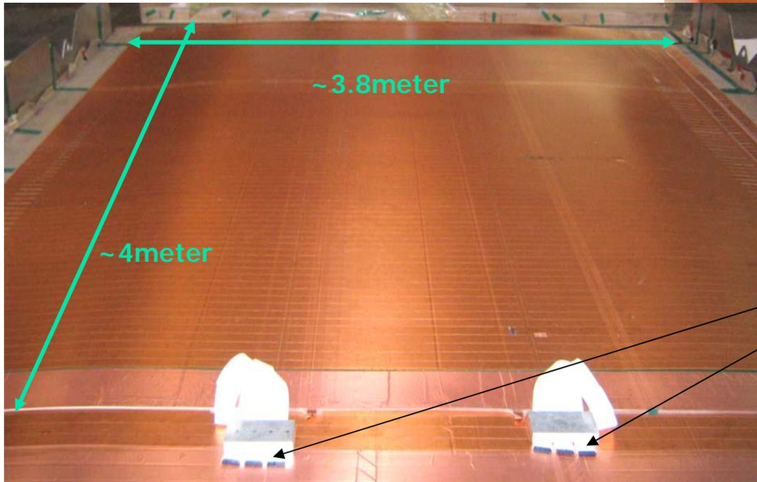
16 channel cables for signal pick up
