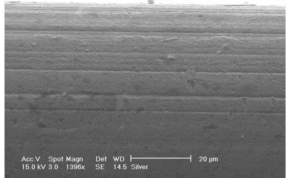
Use SEM scale measured wire diameter is 101μm, micrometer measured is 97 μm.
