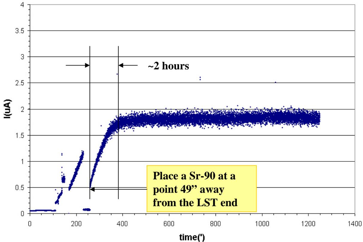
**W/o grounded shielding on the top of LST, under intensive source radiation the anode wire current takes ~ 2 hours to get stabilized.**
