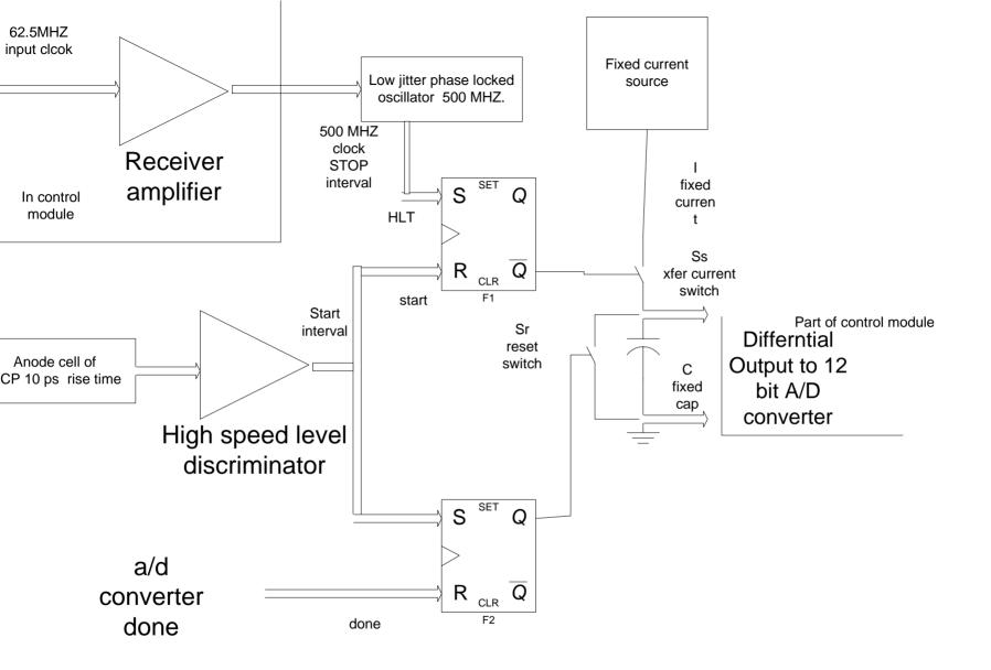
Simplified cell logic 1 Of 4 cells served by control module
