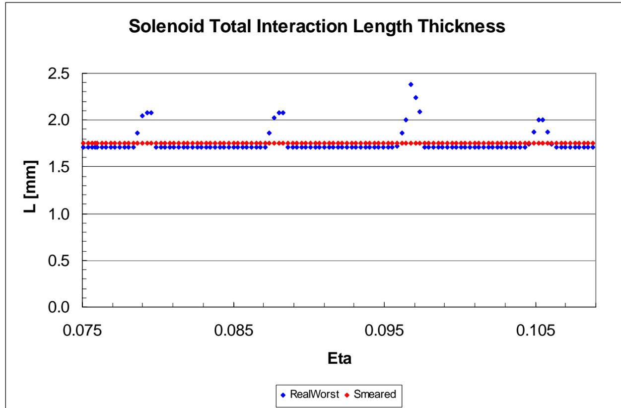
Layers aligned to maximize nonuniformity of conductor
