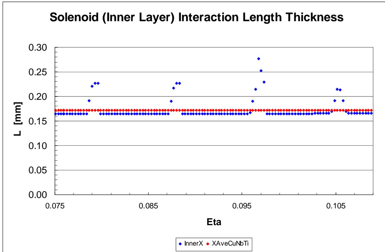
Calculation for single winding layer highlights nonuniformity of conductor
