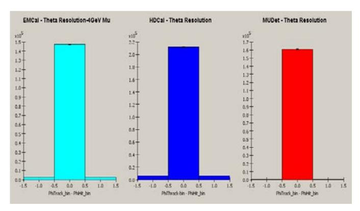
The resolution better ~0.5bin in each detector component, the bin being EMCal(~3.8mrd),HDCal(~5mrd),MUDet(~21mrd)
