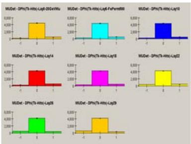
Δφ(Track-Hit) at different radii (layer number) In Mudet for a 20 GeV Muon
