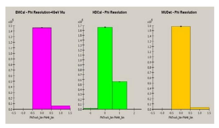
The resolution is better than 0.5 bin in each detector component, a bin being in EMCal(~3.8 mrd), in HDCal(~5mrd), in MUDet(~21mrd)
