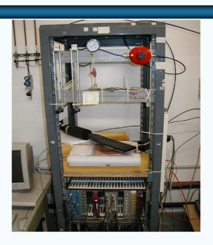
Test 8x8 cm<sup>2</sup> area defined by two scintillator trigger counters.
