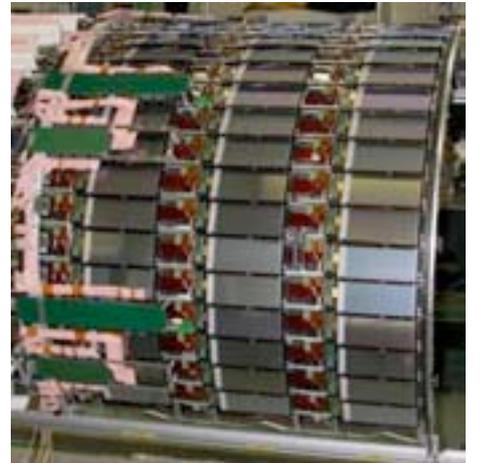
Cathode Strip Chambers on Endcap Muon Disks
