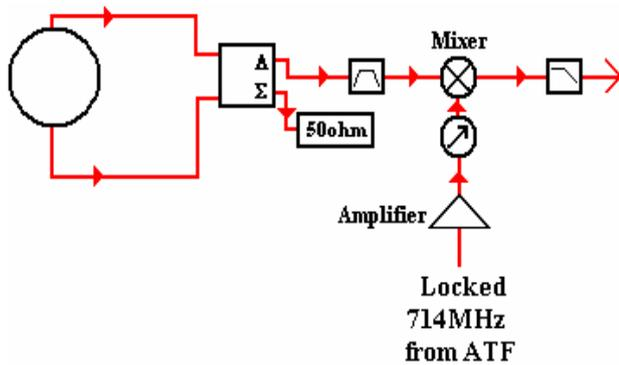
Figure 4: Schematic of BPM signal processor.
