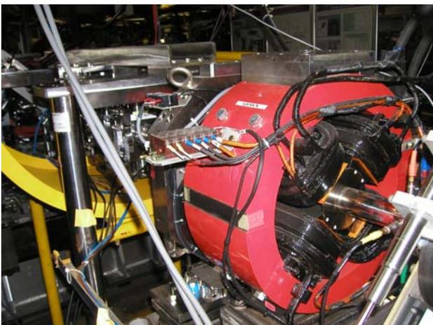
Figure 3: ATF beamline showing the kicker (left) and BPM (right).
