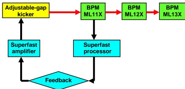
Figure 2: Schematic of the ATF beamline showing location of the kicker, BPMs and feedback system.
