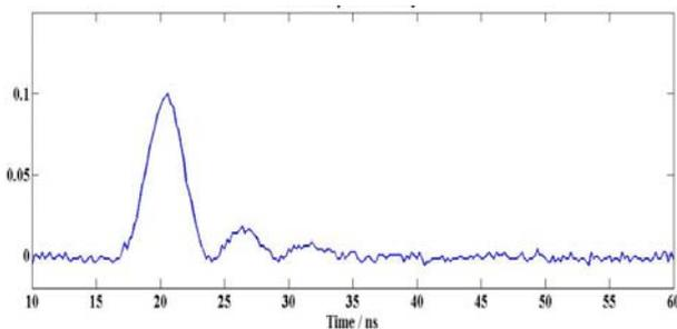
Figure 5: Response of the BPM processor (Volts) to a single electron bunch.
