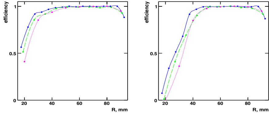
Figure 2: Efficiency to identify 200 GeV electrons as a function of radius in the low (left) and high (right) background regions. Blue full line is for 5 mm cell size, green broken line is for 8 mm and red dotted line is for 10 mm.
