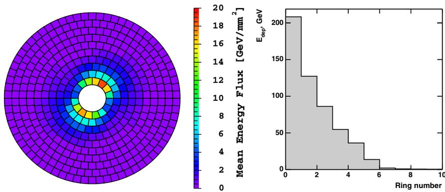
Figure 1: The energy density of beamstrahlung remnants per bunch crossing as a function of position in the  $r - \phi$  plane (left) and the energy deposition in diamond rings as a function of ring number (right).
