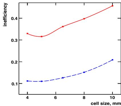
Figure 3: Inefficiency of reconstruction 200 GeV electrons as a function of cell size for the radii below 55 mm. Red full line is for high and blue broken line is for low background region.
