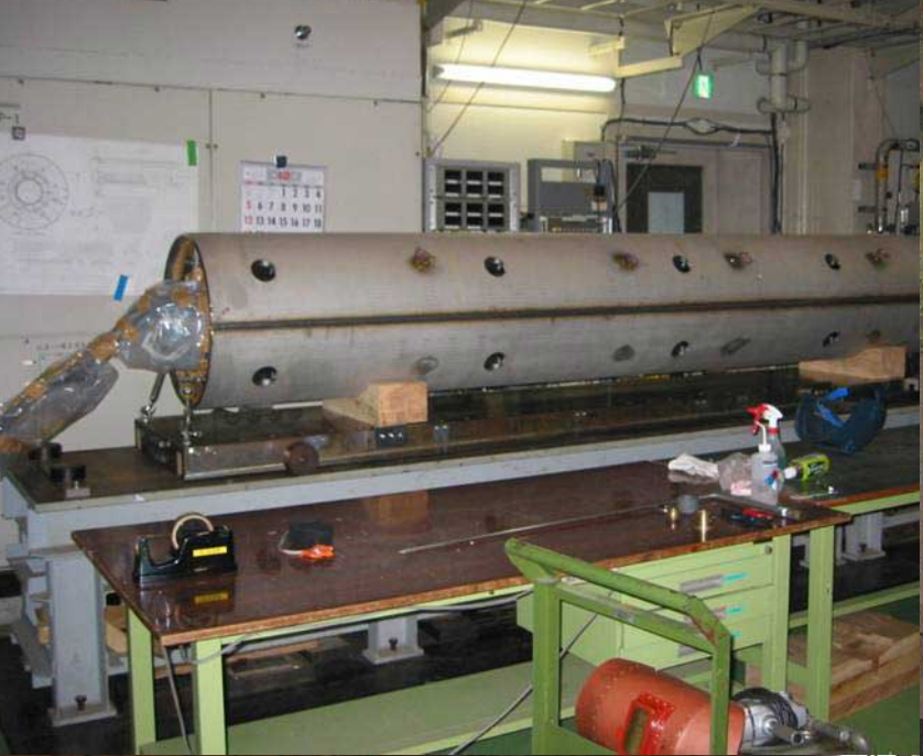
Shell Welding Completed (Dec21,04)
