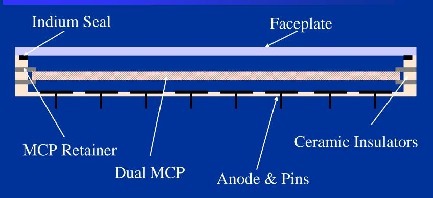
Spacing between faceplate and MCP and MCP and anode can be varied for different applications
