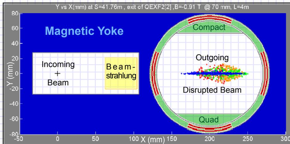
Even if the main part of the disrupted beam and beamstrahlung pass cleanly, there can be synrad hits from upstream magnets.
