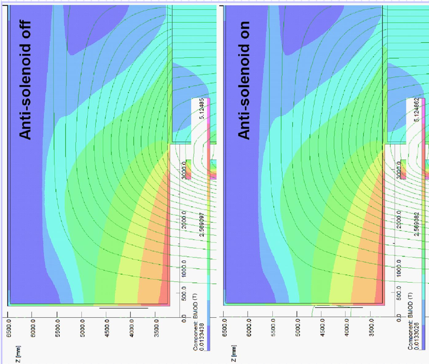
The endcap field is almost unchanged with anti-solenoid ON and OFF.
