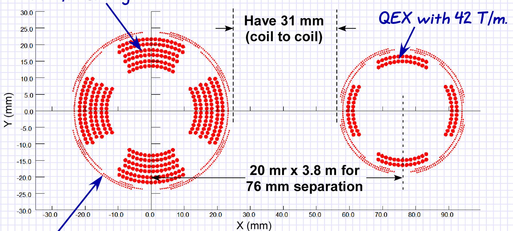
Both magnets have dipole, skew-dipole and skew-quad windings to compensate fringe and detector fields (outbound beam & DID).
