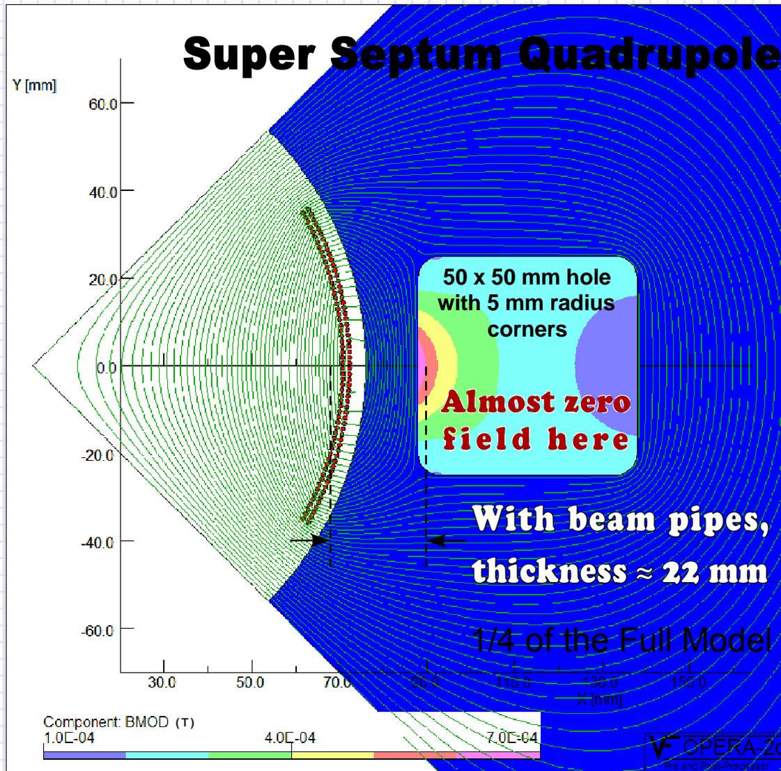
There are places where beams are not well separated but we need to focus one and not deflect the other. This happens frequently along the 2 mr X-ing angle extraction beamline.
