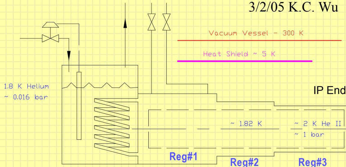
Temp. profile along a channel filled with He II at 1 atm
