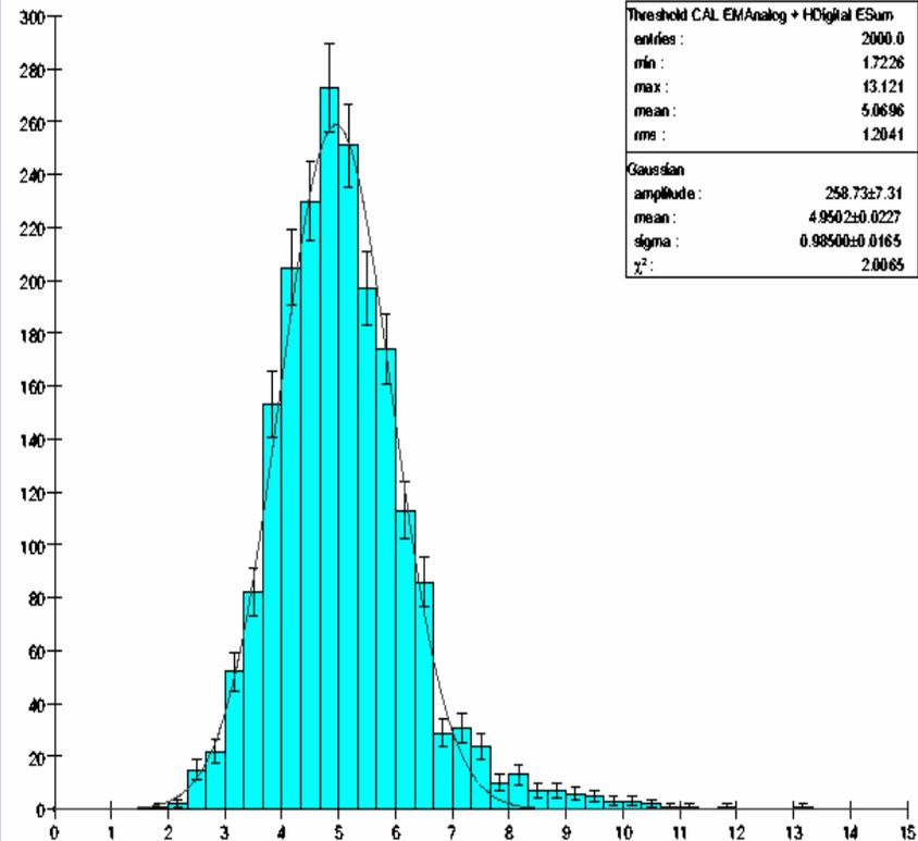
Energy measurement in calorimeter - Analog ECAL, Digital HCAL
