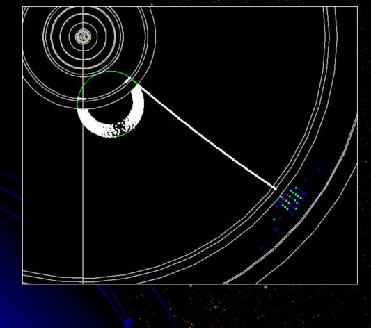
Wired picture of a gamma conversion as simulated by Lelaps for the LCD LD model.
