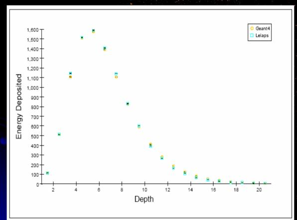
Comparison of CEPack longitudinal profile (green) of a 10 GeV electron in an EM calorimeter with Geant4 (orange).
