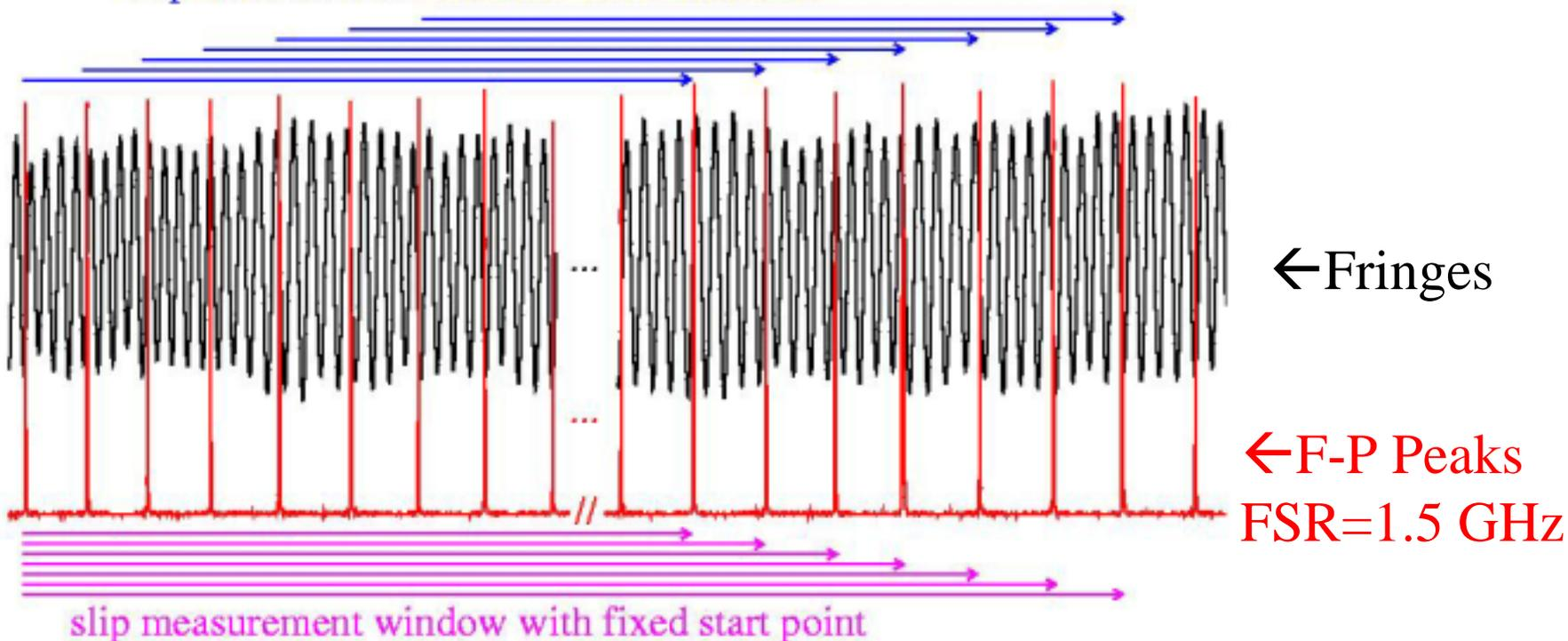
→ If  $t_0$  is fixed, the measurement window size is enlarged one F-P peak for each shift. An oscillation of a set of measured OPD reflects the amplitude and frequency of vibration.
