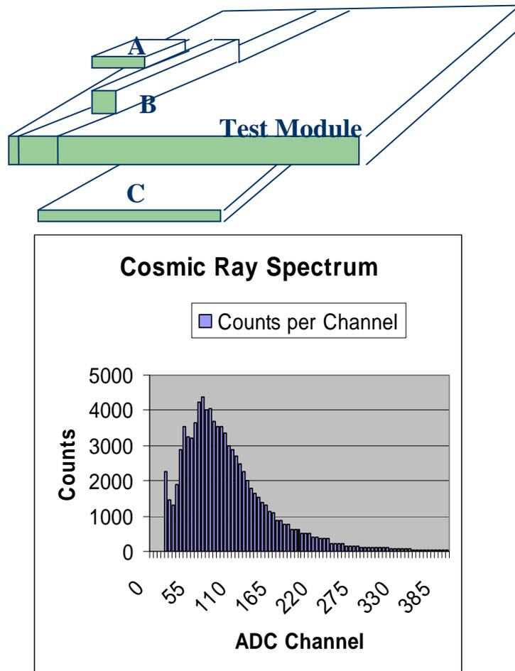
Figure 2. Cosmic Ray Test Setup and Spectrum
