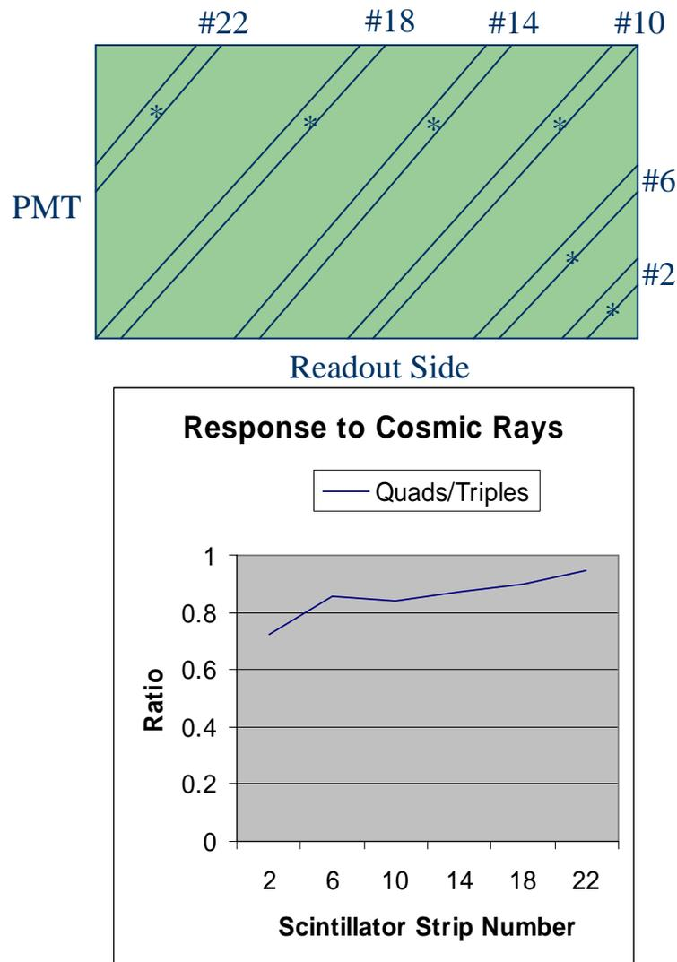
Figure 3. Test Points for Cosmic Ray Tests and Results
