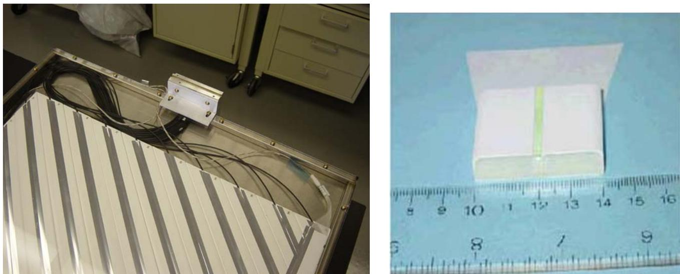
Figure 1. Test Module and cross-section of scintillator strip
