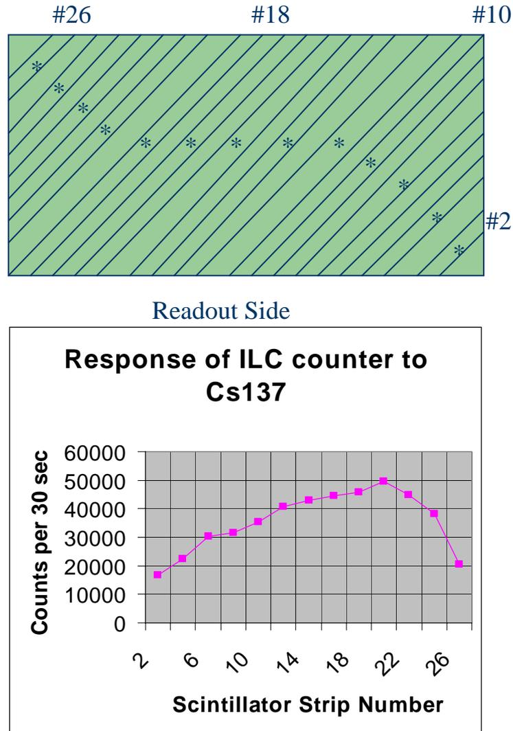
Figure 4. Positions of source and measurements at centers of strips.
